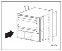
5 Insert and tighten the rack-mounting screws with a Phillips screwdriver.
